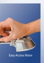
The rotor is designed to hold all standard 1.5/2.0ml tubes (both conical bottom and skirted), and the snap on lid offers space for micro-filter filters that fit into the tops of the tubes. Adapters are available for processing smaller tubes, and our exclusive *StripSpin Adapter* fits onto the top of the rotor for centrifuging standard 8-tube PCR strips.
