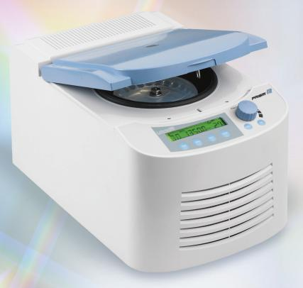
The *Prism's* uniquely designed 24-place rotor allows easy access to the tops of sample tubes, allowing for faster work flow. The individual tube slots in the solid rotor support tubes along their length to eliminate tube deformation or cracking even at the highest speed settings. In the event of a tube failure, tube pieces and samples are contained within the sample well.
